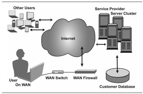
Figure 1.2 End-to-End Architecture View of Streaming Multimedia Content over the Internet
