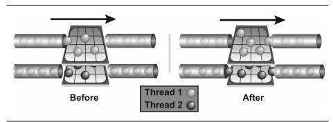
Figure 1.6 Two Threads on a Dual-Core Processor with each Thread Running Independently
